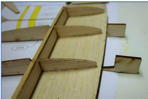
Figure 20: Using Bottom Sheeting Supports
