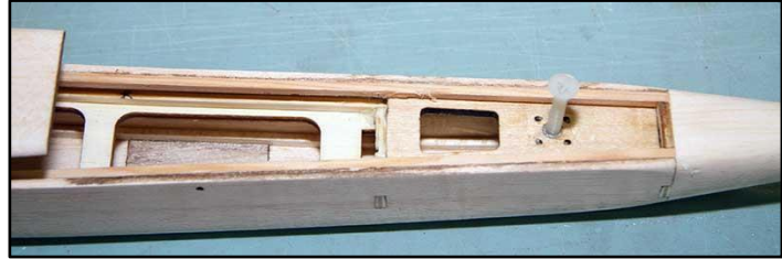
Figure 7: Wing Hold Down Support
