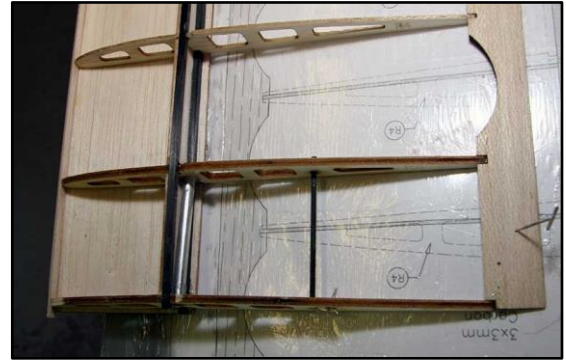
Figure 22: Joiner Tube and CF Reinforcement
